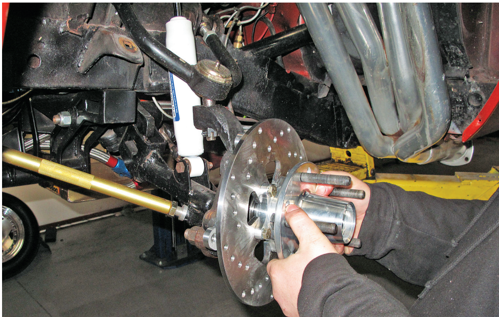
Next, he attached the front caliper brackets (above), and then the rotor was slipped on (left).
