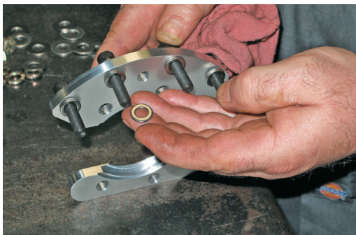
This is the rear caliper bracket, which also retains the axle. The spacers are used to center the rotor in the caliper.
