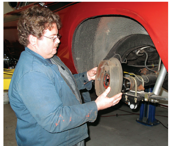
Todd Struck attacked the rear, first removing the axles and then the rear brakes.
