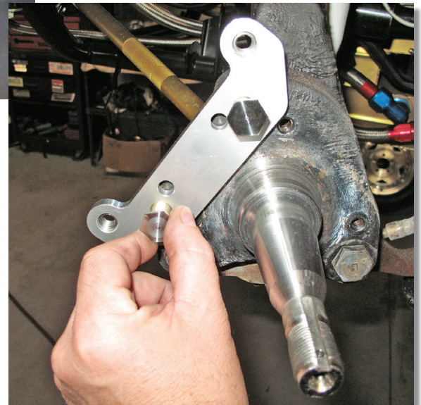
Next, he attached the front caliper brackets (above), and then the rotor was slipped on (left).
