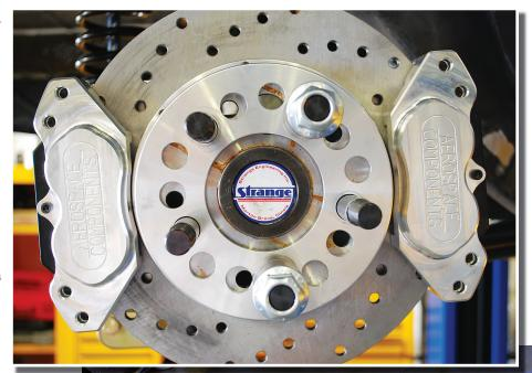
Aerospace Components' dualcaliper rear-brake system will hold your car on the line better than factory brakes, and it should help on the top end as well. A setup like this can help improve staging consistency and elapsed times.
