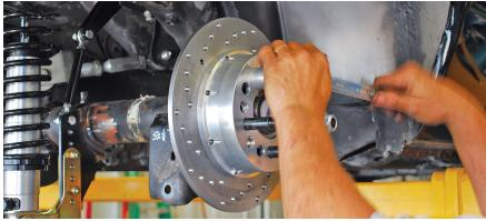
With all three brackets in place, the brake rotors are installed. Two spacers and lug nuts will be threaded onto the study to keep the rotor snug against the axle flanges. Aerospace brake hats are universal and use three-bolt patterns.
