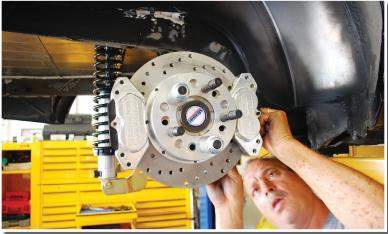
Take the time to line up the second caliper, or pad wear could be inconsistent and drag could result, which will slow you down and increase pad wear. With both calipers mounted, the 90-degree fittings can be installed. Then, the stainless-steel flex lines can be threaded onto the fittings and tightened before joining both lines with a tee fitting.
