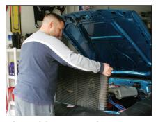
After draining the water from the system, we removed the hoses and the stock radiator. The original Ford piece was factory issued and had about 100,000 street miles and 15 years of ontrack duty. It served its time well but was clogged and not working very efficiently.
