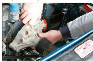
Next, we unbolted the old water pump and cleaned the gasket material from the flange.
