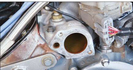
(Above) Most experts agree that it is not necessary in drag racing to run a restrictor in place of the thermostat. The theory is that engine cooling will improve by keeping the coolant in the radiator/engine for a longer period of time, when in fact you want as much flow as possible because this is what removes the heat from the engine. I had a restrictor in place because it was the thing to do but have removed it.
