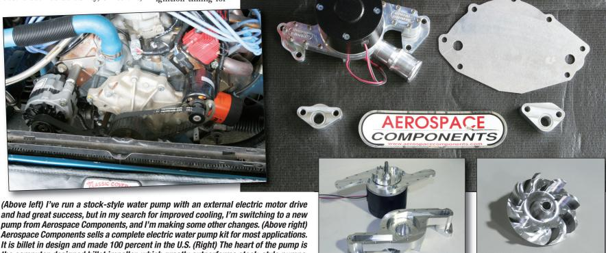
the computer-designed billet impeller, which greatly outperforms stock-style pumps. This unit is designed to flow 37 gallons per minute and can run on 12 or 16 volts.
