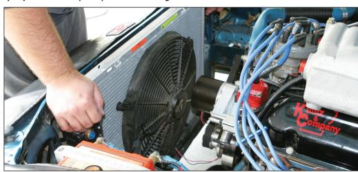
After attaching the electric fan to the new radiator, it was lowered into place. (Note: Before attaching any new fan, test-fit the radiator. This is the second radiator; the first one I purchased from another auto chain did not fit well.)
