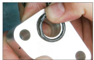
Aerospace supplies two standoffs in the kit to space the pump out. Rubber O-rings seal it from leaks.
