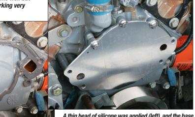
A thin bead of silicone was applied (left), and the base plate for the Aerospace pump was installed (above).
